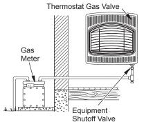
Figure 17 - Checking Gas Joints for Natural Gas
